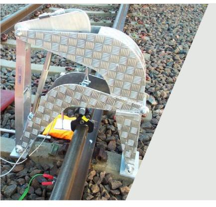
Reducing the risk of derailment as a result of track buckles or rail breaks has long been a priority for railway companies and track engineers. Measuring the stress-free temperature of continuously welded rail is a key part of this, enabling weaknesses and risks to be identified and managed. In the past this was a time-consuming, expensive and often unreliable process that involved cutting the rail.
