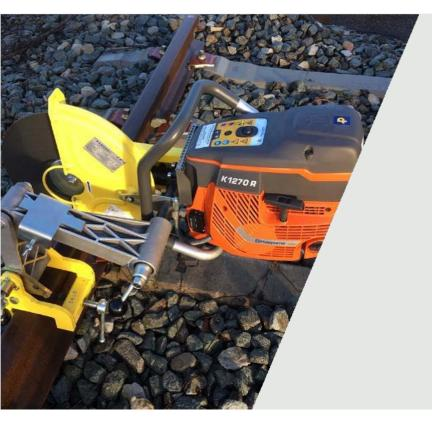
The Pandrol Rail Saw (HC305 / HC355 / HC 406) ensures fast and accurate cutting of rails of all profiles and grades. The ergonomic design of the rail clamp prevents physical stress.
