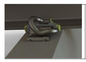
The Pandrol Anti-Theft assembly uses the inherent design of the e-clip as well as a Special designed GPI, to prevent the malicious removal of rail fasting clip from track installations. The Anti-Theft System installs like any other e-clip system but cannot be removed by normal means. The removal requires a modified Pandrol Pan-puller to relieve the toe and heel of the clip, for the clip to be removed. The special design of the GPI allows for the system to maintain electrical insulation.
