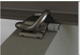
The Pandrol Anti-Sabotage assembly uses the inherent design of the e-clip as well as a Special designed Sleeve, to prevent the malicious removal of rail fasting clip from track installations. The Anti-Sabotage System installs like any other e-clip system but cannot be removed by normal means. The Anti-Sabotage System makes removal of the e-clip extremely difficult and is very effective in areas of track where fastening system removal is problematic.
